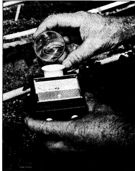
Figure 7. Portable meter for measuring electrical conductivity of nutrient solution.
