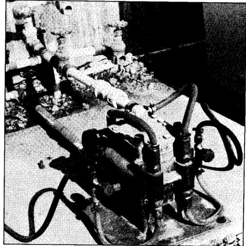
Figure 6. One type of fertilizer proportioner for nutrient-solution feeding.
