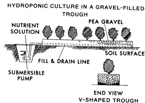
Figure 2. Hydroponic culture in a gravel-filled trough.
