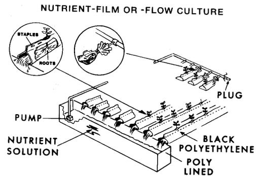
Figure 1. Nutrient-flow culture using plastic film to hold and feed plants through recirculation system.
