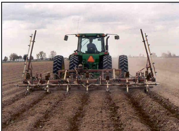
**Figure 14.** A dammer-diker used to make small basins between potato rows to prevent water from running off the field.
