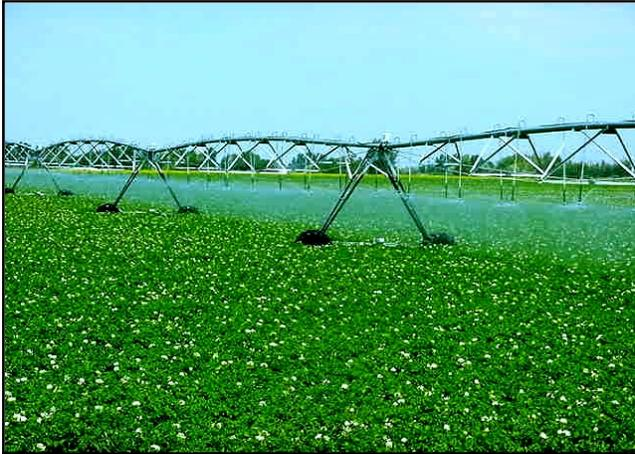
**Figure 16.** A center-pivot sprinkler irrigation system applying water.
